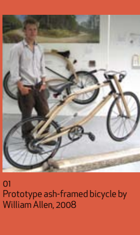
01 Prototype ash-framed bicycle by William Allen, 2008
